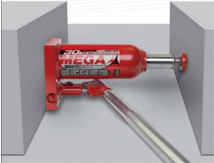
The MEGA jacks can be used horizontally when required. Set the jack with the pump down.
